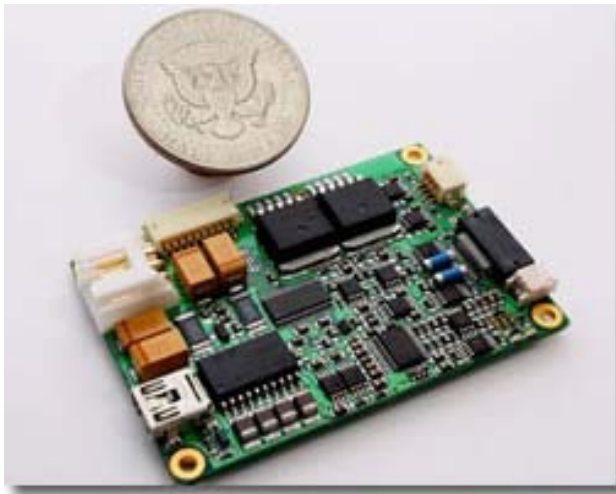
GCU-2K1, Complete DSP based Gyro controller
